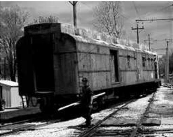
Work continues on Chicago & North Western RPO 8646. The picture on the left shows the car being moved into the shop. On the right, Lowell Diersen rides the side of the car as it emerges from the shop in January, 2009 after undergoing much body work, receiving a new roof, and fresh coat of paint. It's good to see another piece of equipment, which had been deteriorating, undergo such a transformation. Thumbs up to the shop crew for bringing another car back back to life.
